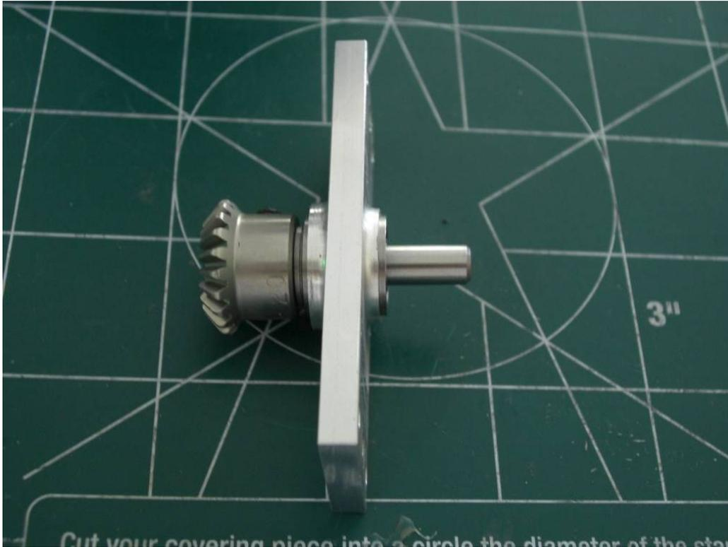
Now mount the gear to the side plates using the 3mm x 8 cap head screws and adjust the gear mesh so there is no backlash and they run perfectly smoothly.
